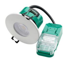
The Firestay Duo LED CCT is a High Output Downlight ideal for high ceilings or any project requiring high intensity light, 4 way colour and 2 wattages switchable straight out of the box. With a 7 year product warranty, the front facing switch enables the user to seamlessly change the colour temperature (2700/3000/4000/6000K) to suit the mood of any space while the rear facing wattage switch enable you to instantly dictate the light level of any commercial or residential premises.
