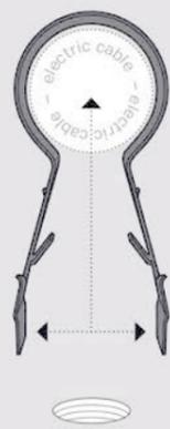
Compress and push it home. Pinch the legs together and push into the hole by hand.
