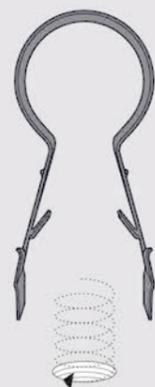
Slide the clip over the cable. Make sure it's seated in the rounded area of the clip.
