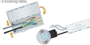
If required, the WAGOBOX 221-4 can be fitted to a surface using the WAGOBOX mounting button feature. (sold separately, part No. 51009130 pack of 10)
