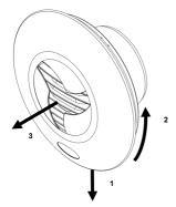
To refit the cover, reverse the above procedure. The iris shutter should be in closed position after refit. If not, wait approximately 1 min after fan switch off allowing the actuator to retract back in the closed position and then refit the cover again.
