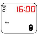
**Step 8:** Press the MENU button. The temperature should flash. Use the + and - buttons to select a frost protection temperature.
