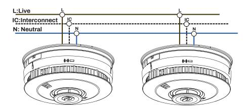
Heat Alarms must always be interconnected to a smoke or multi-sensor Alarm to ensure early warning.
