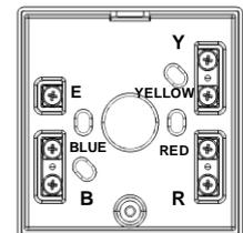
MAGDUO MCPs can be mixed on the same zone as other types of MAGDUO device. The above diagram shows how to make the zone positive, zone negative and screen connections between the control panel and MAGDUO MCPs. Refer to the instruction leaflets supplied with other MAGDUO devices for their equivalent wiring/terminal labelling details.
