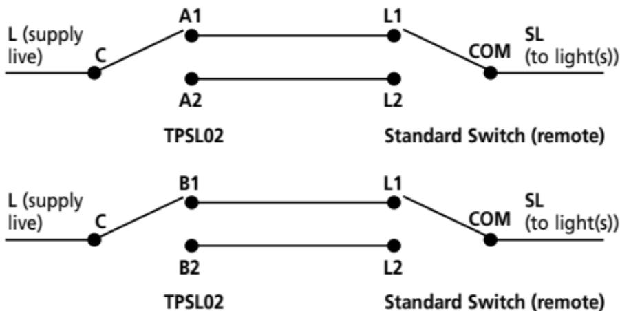
Either standard switch could be a TPSL01 or half a TPSL02). Connections to SL (lights) and L (supply live) can be swapped if required.
